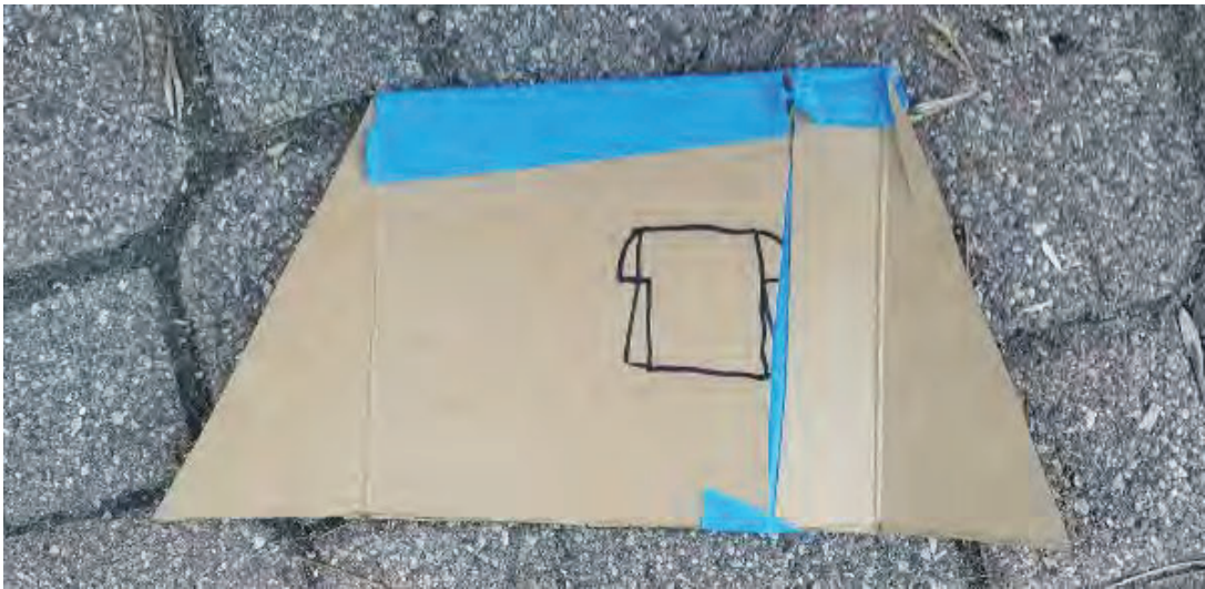
Version 1: too wide and the triangle flaps were improperly cut so the edges interfere with the intake
