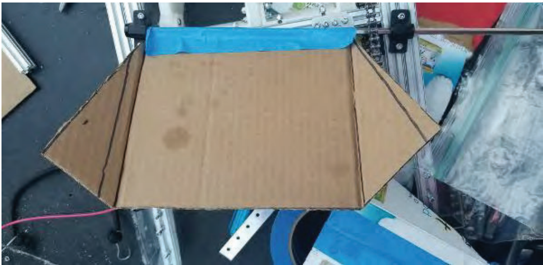
Version 2: fixes problems above, with the hypotenuse of the triangular flaps on the main part of the carrier
